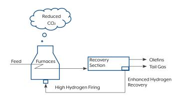
Enhanced hydrogen recovery designs maximize the recovery of hydrogen from cracking process. Recovery section enhanced hydrogen recovery designs, along with hydrogen firing, can be implemented as part of a grassroots cracker development or revamp to an existing unit.
