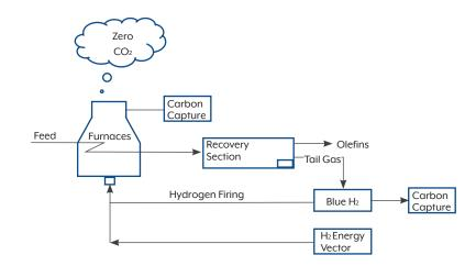
KBR is developing concepts on steam cracking furnace electrification, to completely remove the flue stacks and direct emissions from pyrolysis furnaces.
