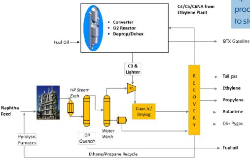
K-COT increases propylene yields, reduces energy consumption and improves liquid crackers' cost of production when compared to steam cracking
