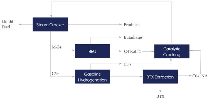
Figure 3: K-COT unit addition for direct conversion of C4+ streams
