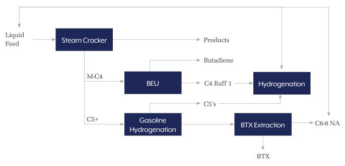
Figure 2: Liquid cracker configuration for C4+ streams recycle
